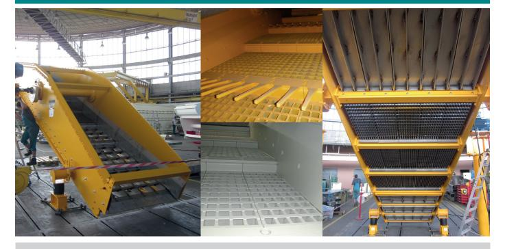
With BIVITEC, Binder+Co starts where conventional screens become inefficient and less economical. Difficult products, such as damp, stalky and leafy materials or matted substances block the screen openings of conventional screening machines and thus make efficient screening impossible.
